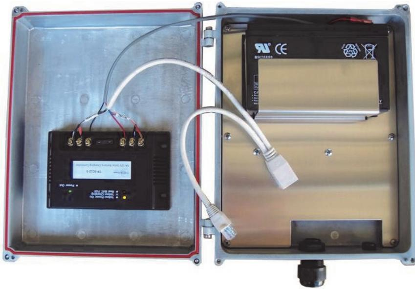
**STEP 1:** Connect Battery to Controller. Be sure to observe polarity. Black wire connects to battery negative terminal. When battery is connected the yellow power-on LED should light on controller.
