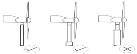
**Figure 2: Blade and pole clearance**
