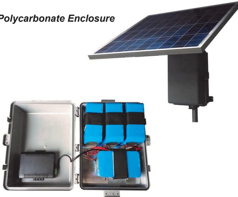
**STEP 2:** Mount the enclosure. We recommend mounting the enclosure under the solar panel so that the enclosure is shaded from peak summer sun. This will help prevent excess heating of the enclosure during summer months. Be sure to mount just low enough that when you open the door, it will clear the panel.
