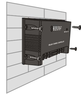
4 screws are provided for mounting purposes. Please ensure both cooling vents on either side of the controller are free from obstruction to ensure sufficient air flow.
