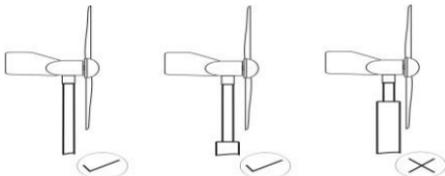
**Figure 3: The clearance between the blade and pole**
