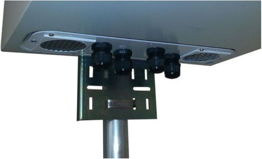
**STEP 4:** Route red and black wires to a 12VDC /24VDC power source. Connect red wire to V+ and black wire to V-.
