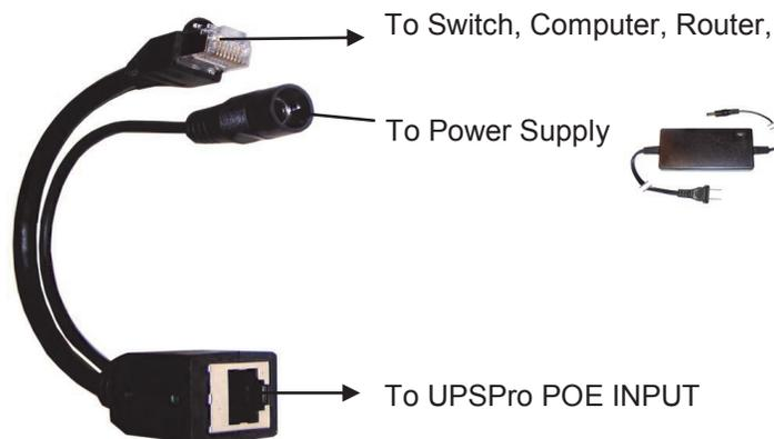
**STEP 3:** Connect your equipment to the 12V POE Output connector or back wire terminal connector as desired. Connect the green connector to the controller. The LOA LED on the controller should light.
