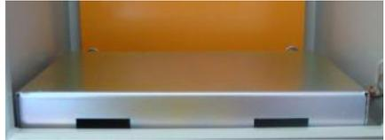
**STEP 7:** Attach the Green DIN Rail adapters to the charge controller using the screws provided. Use 1 screw per adapter. Clip the controller to the DIN rail.
